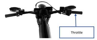
Before each use, check that the throttle grip rotates and returns correctly to prevent any accident.
