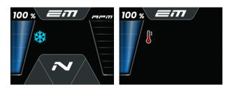
These temperature indicators appear when the battery temperature is below 10°C (Snowflake) or above 55°C (Thermometer).
