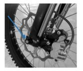
Compress the fork gently (approx. 3 to 4 cm) and repeat the operation 2 to 3 times to center the wheel axle.
