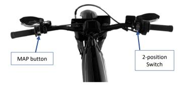
On the right side of the handlebar, the ON position of the security switch is needed to switch on the motorcycle.
