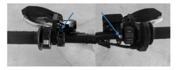
For the lever positionning, you have to adjust these 2 screws
