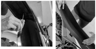
Remove the main cover by en spreading the sides
