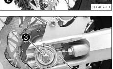
Clean and grease wheel spindle 1.
