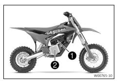
The LV traction battery 1 is air-cooled.
