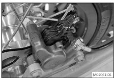
Put the new brake lining in position.
