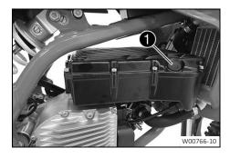
The On/Off button 1 is located on the right side of the LV traction battery.
