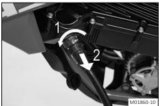
Unlock the charging plug lock counterclockwise and disconnect the charging cable from the LV traction battery.
