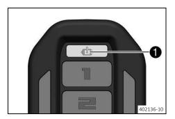
The malfunctions are indicated by malfunction indicator lamp **1** and by acoustic signals that sound at the same time.
