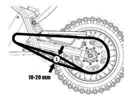
Rotate the rear wheel moving the tire with your hand, stopping at different positions to check the chain's clearance, always taking the measurements in the same place.
