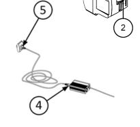
The LED 2 will turn green when the battery is fully charged. It will take about 4 hours to fully charge in the case of a series ONE battery, and 5.5 hours for a full charge in the case of a KIDS TWO series.
