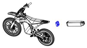
maximum capacity. To connect it for the first time, and after each ride, the battery must be removed as explained in the <u>Charge the battery outside the vehicle</u> section and the foam spacer that is between the battery connector and the battery compartment should be removed.
