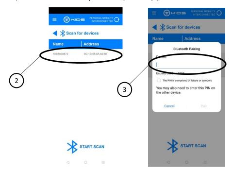
5. If the mobile has already been paired previously with the Bluetooth device, this step will not be required given that the pairing will be done automatically, and you could act directly in the main menu. Once the smartphone has been paired with the motorcycle's Bluetooth device, the message "Device Connected!" (4) will appear at the bottom of the main menu.
