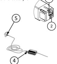
The LED will turn green when the battery is fully charged. It will take about 3 hours to fully charge in the case of a series ONE battery, and 4 hours for a full charge in the case of a KIDS TWO series.
