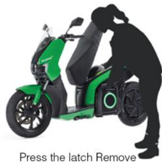
Press the latch Remove the battery pack
