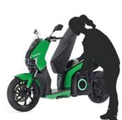
Press the latch Remove the battery pack
