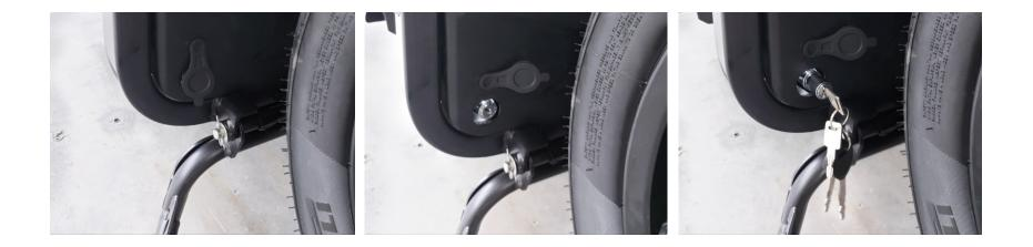
**IMPORTANT:** Never remove or insert the battery pack when the scooter is charging or with the key in the ignition. Make sure **not to unfold the handle before pulling the pack out** (unfold it after the battery has been removed from the scooter).
