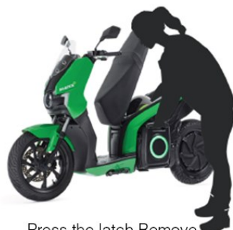
Press the latch Remove the battery pack
